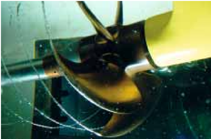
■ Fig. 1 – Propeller model during testing at BVT’s cavitation tunnel in Portsmouth.
